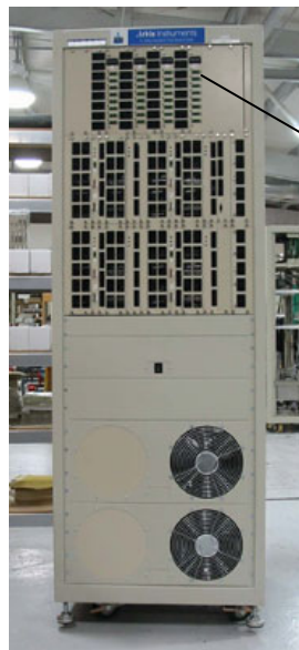
4-channel BT2000, 5V/40V, 50A/5A/1A, 2kW max with 4 equalizer modules of 8-channel each for testing 10-cell lithium battery pack.
