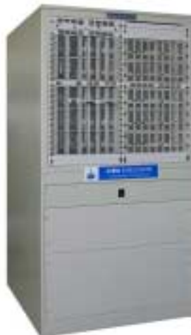
A one-channel linear charge-discharge testing system of 60V, 150A, 9000W with three-current ranges 150A/50A/1A. The one channel is constructed from 10 individual channel boards with one serving as the master. The size of the system is 78"H x 25"W x 28"D.
