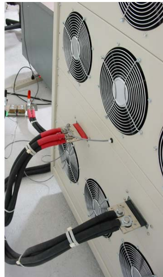
1-channel linear battery testing system of 2500A/1A, 6-36V, and max 30kW power. Maximum discharge current at 2500A within power limit.
