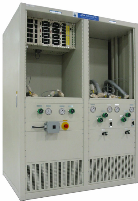
A 3-channel combination PEM/DM fuel cell testing system. Left unit for PEMFC, right unit for DMFC testing.
